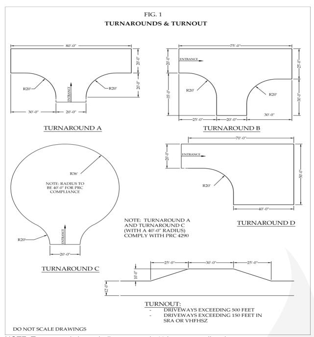
NOTE: Turnaround slope shall not exceed 5% in any one direction.
