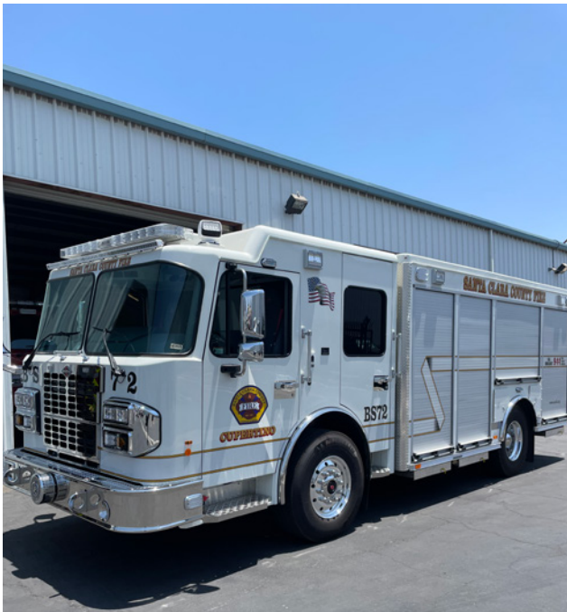
A new Breathing Support Unit (BSU) replaced an end-of-life unit that joined the fleet in 2005. The BSU transports critical self-contained breathing apparatus (SCBA) bottles and has a mobile air compressor to refill multiple bottles simultaneously on scene of incidents.
