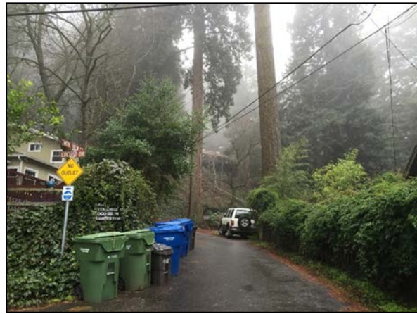
Figure 1-1.9. Dead-end spur road in Redwood Estates showing narrow road width and obstructions to emergency vehicles.
