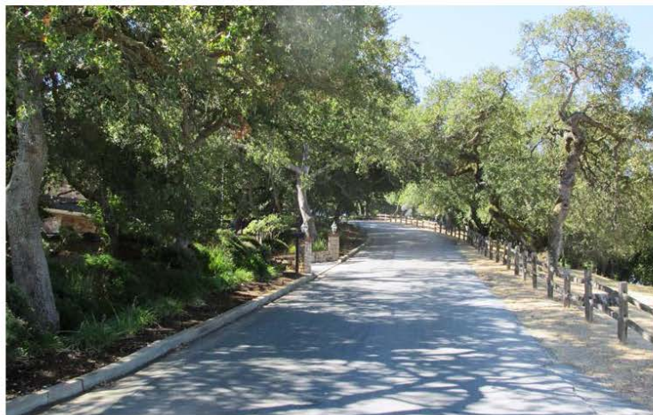
Photo 23. Effective 10' fuel break on both sides of roadway.
